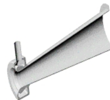
b) Section throughout a Coandă ejector
